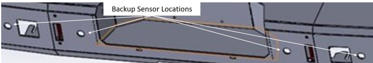
Figure 9: Rear Chevy 3500 backup sensor locations
